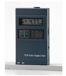
roughness profile and its mean line, or the integral of the absolute value of the roughness profile height over the sampling length.
