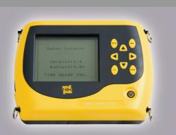
Detection of rebar and other metal building elements (such as steel pipes) and their orientation
