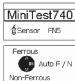
Now the gauge is in the **measure mode** (see fig.) and ready for measurement. The **measure screen** appears. Readings are not yet available.
