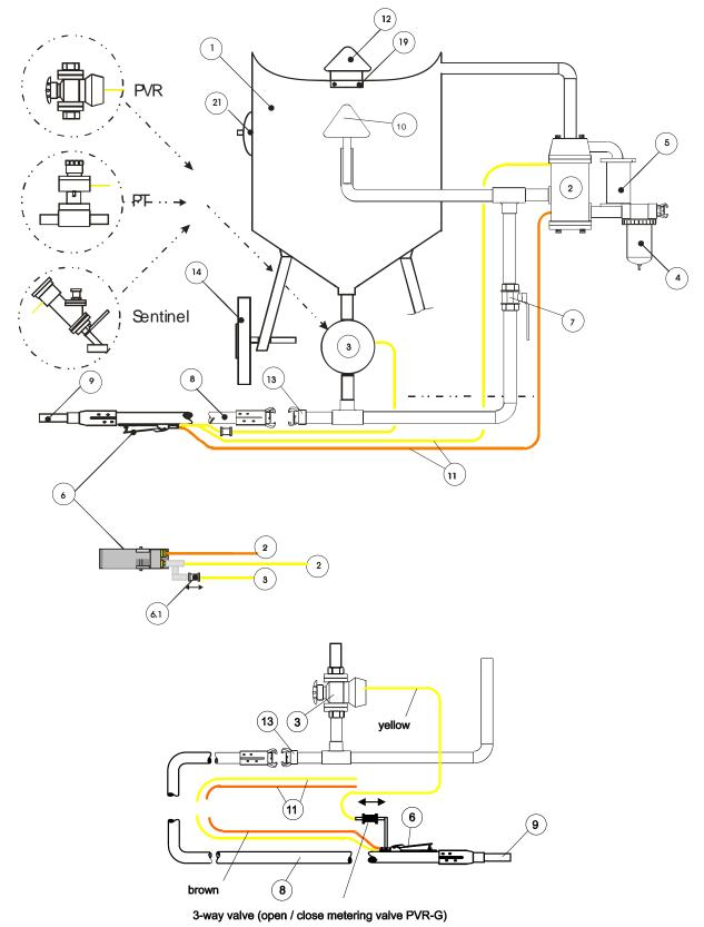
Figure 4: Dual function pneumatic.
