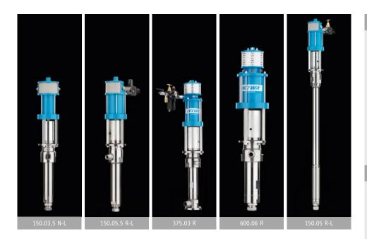
**These new low pressure pumps** still use the well proven WIWA compressed air motors. The transfer pumps differ from their predecessors by the following features: Revolving piston gland packing with four V-sleeves, easy assembly and disassembly, low weight, the piston is simply hooked in, as with the Airless paint spraying units.
